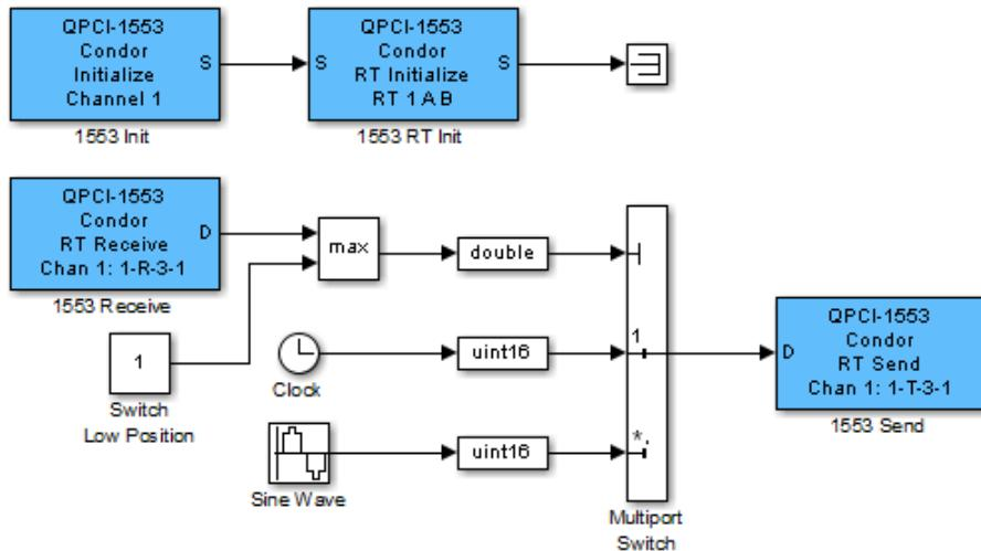
The QPCI-1553 Initialize block configures the board for Remote Terminal operation on channel 1 of the board. The QPCI-1553 RT Initialize block configures the Remote Terminal 1 to monitor buses A and B for incoming messages and configure the active transmit and receive sub addresses. The QPCI-1553 Receive and Send blocks use sub address 3 for both transmit and receive. Note the message parameters notation 1-R-3-1 on the QPCI-1553 Receive and Send blocks. This notation has the format:
