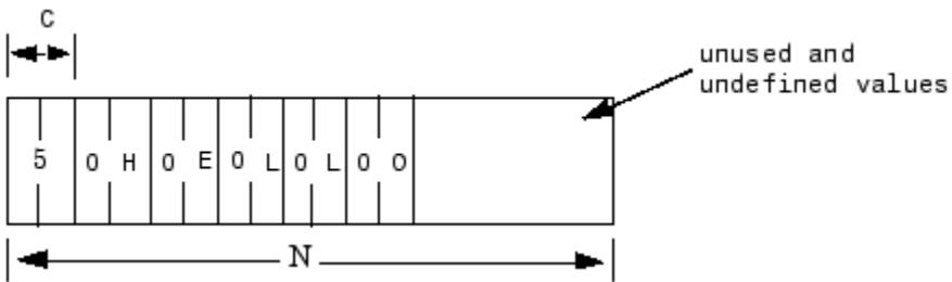
These serial blocks interpret each entry in the vector as a single character. The low-level hardware Send block writes the low-order byte of each entry to the UART. The 16- and 32-bit data types allow the embedding of 8-bit data values, including 0. The 8-bit data type is most useful with the ASCII Encode and Decode blocks. The 16- and 32-bit data types are most useful for binary data streams.
