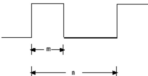
For a base frequency  $b$ , this results in a rectangular output signal of frequency  $b/n$  and duty cycle  $m/n$ . Because  $m$  and  $n$  must be integers, it is not possible to provide a continuous range of output frequencies and duty cycles with perfect exactness.
