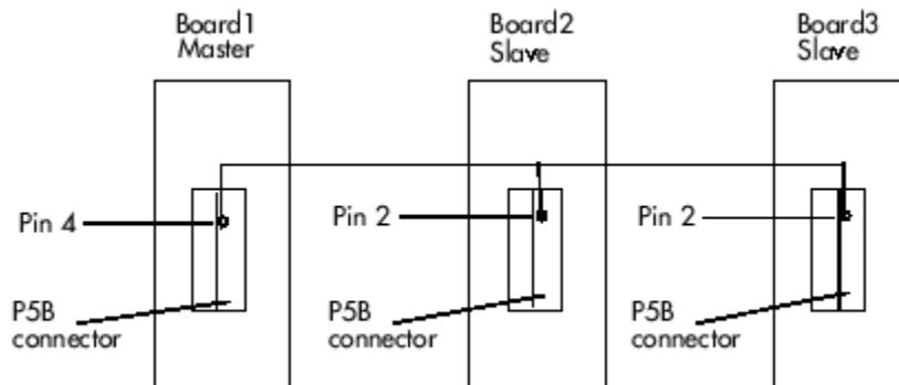
**Note:** The pulse of the master board INPUT TRIGGER READY output occurs 250 nanoseconds after the software trigger in the A/D Start block. This results in a 250 nanosecond delay, relative to the master board, for the slave boards, but should still be considered simultaneous in most situations.
