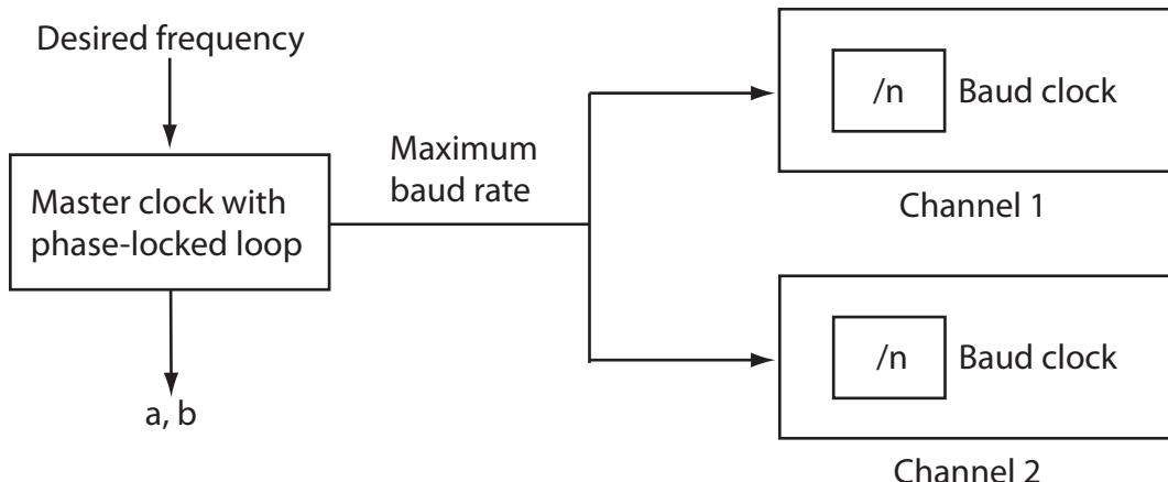
To set the block parameters for this board, choose a maximum baud rate, as follows. This procedure assumes that both channels require different baud rates. Determine a common base clock that can be divided to produce the required baud rates for both channels, as follows:
