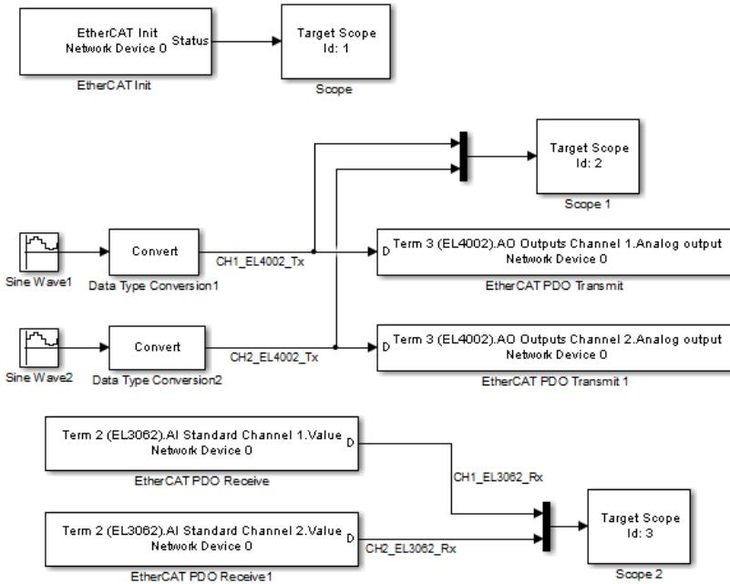
To configure model `xpcEthercatBeckhoffAIO` for execution using the target computer as master node, execute the following steps. You must have used the Beckhoff ET9000 EtherCAT Configurator program to configure the network.
